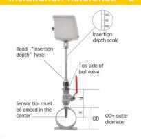
Correct Installation The sensor tip must be in the center of the pipe / tube.
